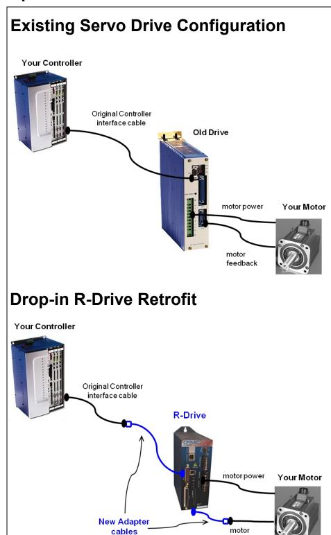
The R-Drive efficiently replaces existing Servo Drives and interfaces to current controller applications.
