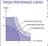
**NOTE:** Continuous torque specifications obtained with motor mounted to an 10''x10''x.25'' aluminum plate at 25 C° ambient. Typical values are within  $\pm 10\%$  of rating.
