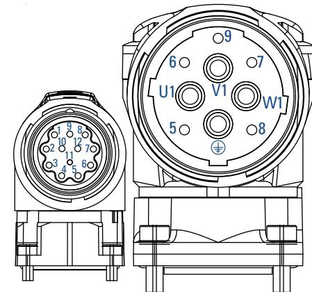
**Resolver Connector      Power Connector**
