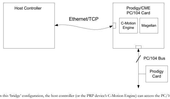
Figure 2-5: Host Controller & Magellanattached Devices
