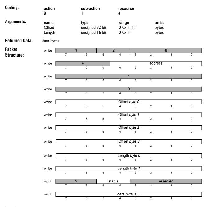
**Description:** The **Read Word Peripheral** action is used to read a sequence of 16 bit data words from a peripheral associated with a PC-104 ISA bus. The **Offset** argument is an offset from the base address that was specified when the peripheral was opened; **Offset** must be even. The *Length* argument specifies the number of bytes to read; **Length** must also be even. The data read is returned as the message body of the response packet.
