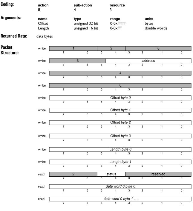
**Description:** The **Read DWord Memory** action is used to read a sequence of 32 bit double words from a random access memory. The **Offset** argument is an address in the memory, typically an address in a dual-ported RAM. **Offset** should be divisble by four, the results of reading from a non-aligned address are unpredictable. The **Length** argument is the number of double words to read, exactly this number of double words are returned as the message body of the response packet.
