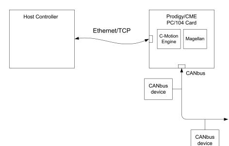
Figure 2-2: Example Network Configuration
