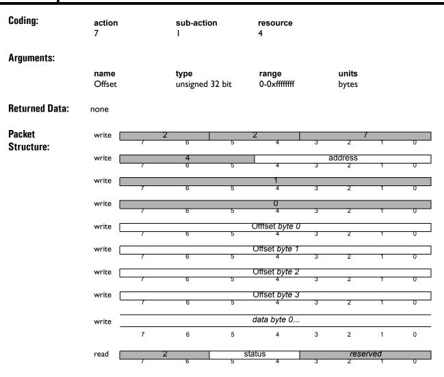
**Description:** The Write Byte Peripheral action is used to write a sequence of data bytes to a peripheral associated with a PC-104 ISA bus. The *Offset* argument is an offset from the base address that was specified when the peripheral was opened. As many bytes as are supplied in the packet are written to the ISA bus from the address given by the base address plus *Offset*.
