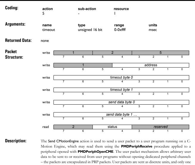
packet may be buffered before being read by a user program. The *timeout* argument specifies how many milliseconds to wait for the user program to read the user packet. A *timeout* value of 65535 (0xffff) means no time limit.
