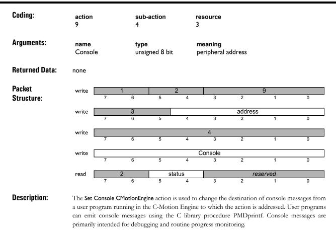
The **Console** argument is the address of a peripheral to be used for console output. If **Console** is zero, then all console output will be suppressed. If **Console** is nonzero it must be the address of a peripheral that was opened on the same device as the C-Motion engine being addressed – if it is an inappropriate peripheral address then an error will be returned.
