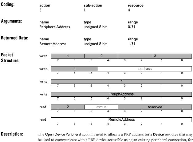
**ESCRIPTION:** The Open Device Peripheral action is used to allocate a PRP address for a **Device** resource that may be used to communicate with a PRP device accessible using an existing peripheral connection, for example a TCP or serial connection. The **RemoteAddress** returned may be used for any PRP action that may be addressed to a **Device** resource; it is typically used to obtain addresses for remote motion processors, dual-ported RAM, and C-Motion engines.
