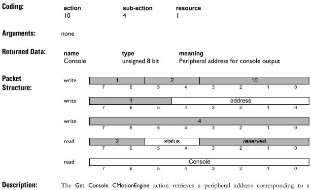
**escription:** The **Get Console CMotionEngine** action retrieves a peripheral address corresponding to a communications channel used for output of debugging and diagnostic messages by C-Motion user programs. The result of this action may not be meaningful if the console output was initially **Set** from a different device than the **Get** is issued from.
