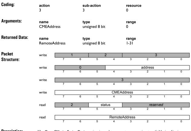
**Description:** The Open CMotionEngine Device action is used to request a connection to a C-Motion Engine on a remote PRP device. The *CMEAddress* argument indicates which *CMotionEngine* resource on the remote device is to be used, for current PRP devices there is only one, so its address is always zero.
