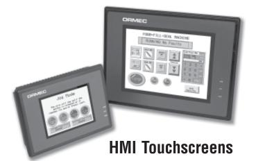
Cost-effective, standalone touchscreen HMIs utilize Modbus RTU (Serial) or Modbus/TCP (Ethernet) communications. Or you can utilize Windows-based HMIs such as Wonderware InTouch, Rockwell Automation RS View, Intellution iFIX, CiTect or GE Cimplicity that communicate with the SMLC using an OPC Server. See page 13 for more information.
