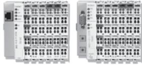
Conserve panel space by utilizing Modbus/TCP (Ethernet) or Profibus DP to connect up to 512 I/O per bus coupler and thousands of I/O points.
