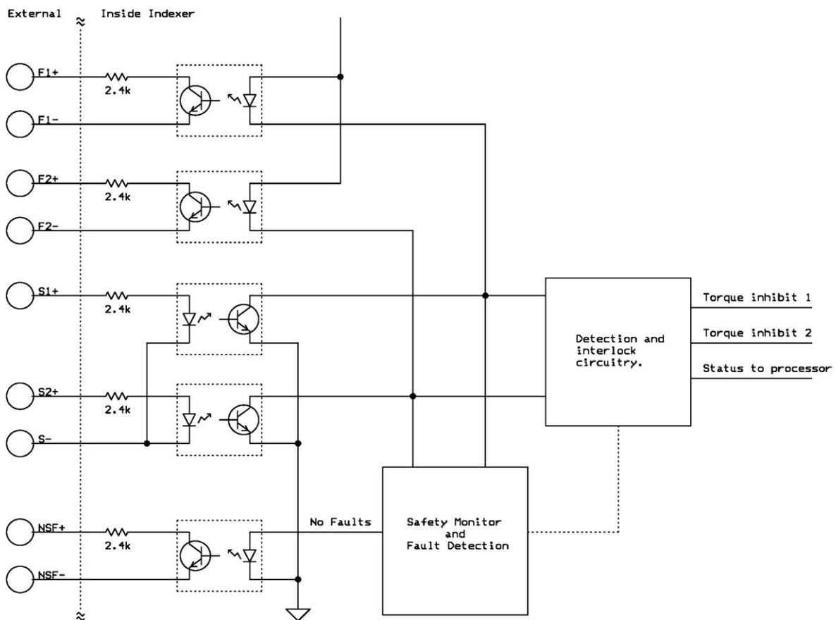
Figure 2: Simplified Safety Circuit Diagram
