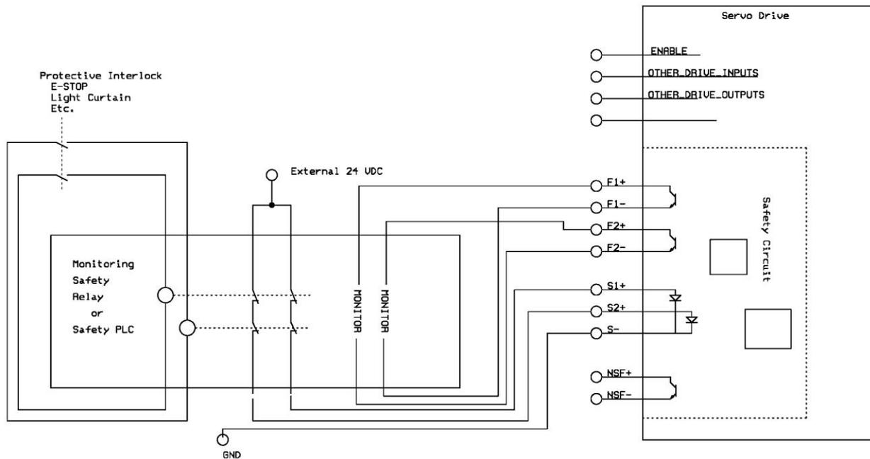
Figure 3: Typical connections for Category 4 installation
