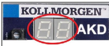
AKD fault codes or warning codes are displayed constantly if present. Fault messages are coded with "F", warnings are coded with "n". With built-in I/O option card, SD card operation errors are displayed with "E" followed by 4 digits.
