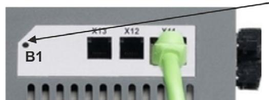
The display shows **En** during the process of changing DRV.TYPE to EtherCAT.
