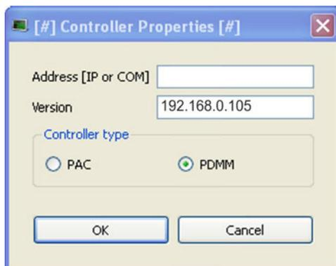
Type in the IP address of the AKD PDMM, set the **Controller Type** to PDMM and click OK. To connect to the PDMM, download, and run the project use the following controls:
