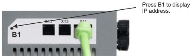
You can use the rotary switches to set the IP address of the AKD. For CANOpen and some other fieldbuses, the rotary switches also set the node address of the drive for that specific network.
