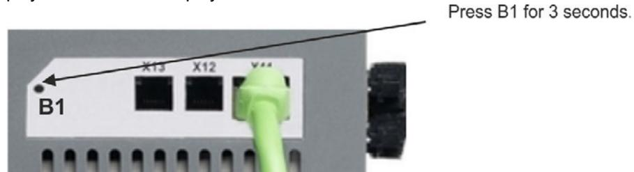
3. When the display blinks with the set rotary switch setting stop pushing B1 and wait until the blinking stops. During that time the parameter FBUS.PARAM01 is set to the new value and all parameters are stored to the non volatile memory. The new setting will be taken with the next power-up of the drive.
