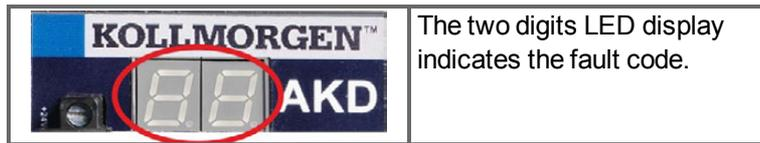
The additional runtime fault messages for AKD-T are coded with numbers starting from F801. All faults activate the fault relay and can be cleared with `DRV.CLRFAULTS`.
