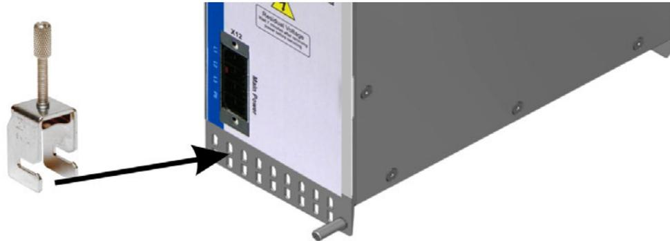
We recommend using Phoenix Contact SK14 shield clamps with clamp range of 6 to 13mm. The clamps hook into the grounding plate and ensure optimum contact between the shield and the grounding plate.
