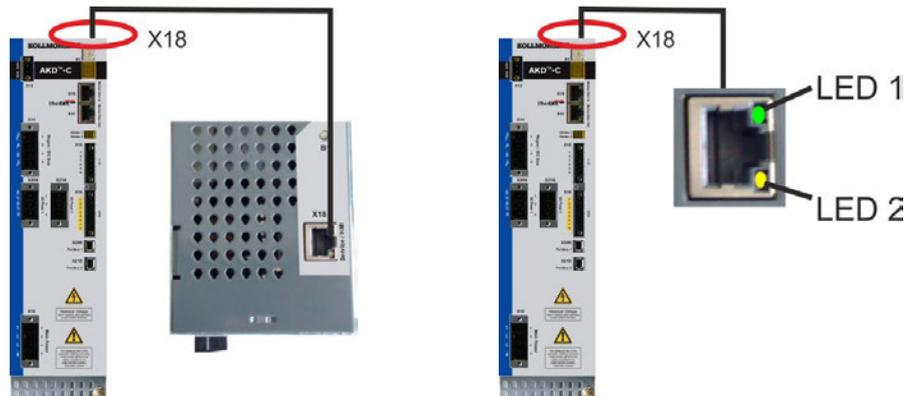
Connect the service interface X18 to an Ethernet interface on the PC directly or via a network switch. The cable can be connected/disconnected to X18 with power on. Confirm that the link LED on the AKD-C (the green LED on the RJ45 connector) and on your PC (or network switch) are both illuminated. If both lights are illuminated, then you have a good electrical connection.
