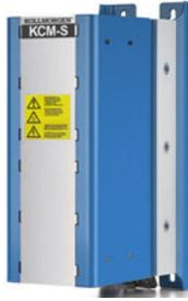
**KCM** modules (**K**OLL**M**OR**G**EN **C**apacitor **M**odules) absorb kinetic energy generated by the motor when it is operating in generator mode. Normally, this energy is dissipated as waste via regen resistors. KCM modules, however, feed the energy they have stored back into the DC Bus link as and when it is required.
