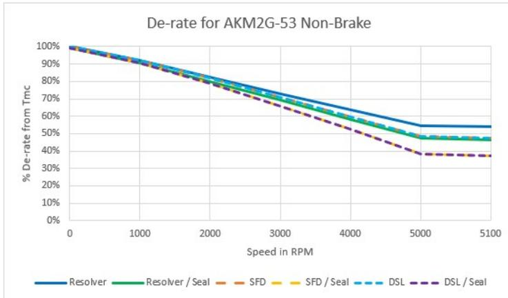
De-rates are referenced to the Max Continuous Torque  $\Delta T$  wdg. = 100°C
