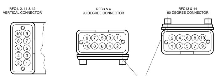
REMOVE THESE SCREWS ONLY IF ABSOLUTELY NECESSARY. IF REMOVED, ENSURE CONNECTIONS ON U/SIDE OF CONNECTOR ARE ALTERNATIVELY PROTECTED FROM CONTACTING CONDUCTIVE OR ABRADING SURFACES.
