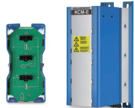
The energy reserves can increase almost unlimitedly with the expansion modules KCM-E. A discharge resistor is integrated into every module. The connection is made to connectors on the top side of the module using the cable protected against polarity reversal that is supplied.
