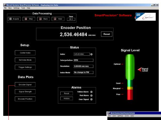
SmartPrecision Software makes Mercury the industry's easiest to use encoder. It helps you program, set up, use, and diagnose Mercury 3500Si encoders with the click of a mouse. Compatible with Windows 95, 98, ME, NT, 2000, and XP.
