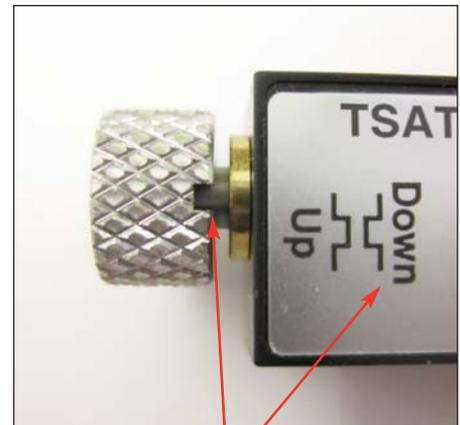
Close-up of plunger knob in the DOWN position. Position of notch indicates that the plunger is in the DOWN position.
