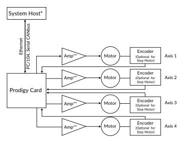
\*System host optional for Prodigy Programmable PC/104 and Stand-Alone cards \*\*External amps used with non-Machine Controller card
