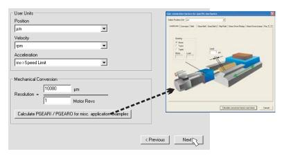
The user units for all input fields in the setup software can be preselected here.
