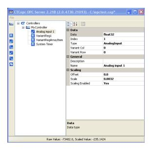
Note above where scaling is enabled on an AnalogInput. The value read from the controller of -73482 (Raw Value) is multiplied by .0032 yielding a result of -235.1424 (Scaled Value). Although the controller represents the AnalogInput as an integer, the OPC Client will see a VT\_R4, floating point, representation of the data with a value of -235.1424.
