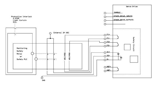
Figure 3: Typical connections for Category 4 installation
