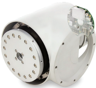
Figure 10: Collaborative Robot Axis Joint with Integrated Safe Electronics
