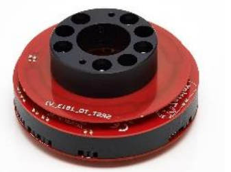
Electrically duplex lightweight encoder with collar clamp.
