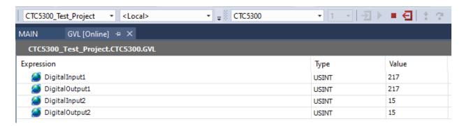
The digital outputs will start incrementing and if a loopback connector is in place the digital inputs will increment as well. Click the red stop icon to stop the program and the red left facing arrow to log off interacting with the PLC. Reference TwinCAT documentation for additional details.
