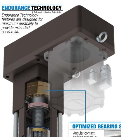
The RSX096P press actuator expands the extend force capability to 40,000 lbf (178 kN) making it well suited for applications such as pressing, riveting, clinching and many others. The RSX096P press model has all the features of the standard RSX on pages 4 & 5 plus oversized tie rods, a bearing system optimized for high force extend, and a high strength steel front flange.
