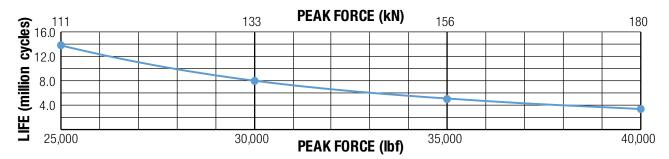
**NOTE:** The L10 life estimation method does not include failures caused by other conditions such as contamination, misalignment, improper lubrication and exceeding actuator specifications
