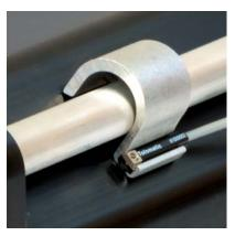
RSX actuators offer a wide range of sensing choices. There are 12 switch choices: reed, solid state PNP (sourcing) or solid state NPN (sinking); in normally open or normally closed; with flying leads or guick-disconnect.
