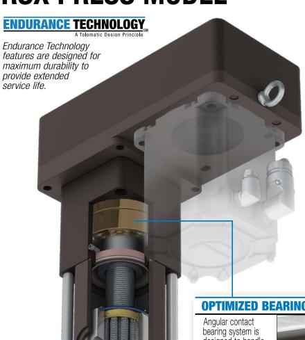
The RSX23P & RSX33P press actuators expand the compression force capability to 23 & 33 tons (46,000 & 66,000 lbf) making them well suited for applications such as pressing, riveting, clinching and many others. These press models have the same features as the standard RSX on pages 4 & 5 plus oversized tie rods, a bearing system optimized for high force extend, and a high strength steel front flange.
